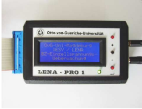
Fig. 4. Developed voltage control with technical data. Number of measuring points = 32; voltage range = 0–1024 V; resolution = 10 bit; sample rate = ca. 10 Hz for all 32 cells; interface = RS-232; supply voltage = 4–26 V dc ; minima = 3U_{\min} with cell number; moving mean = 4 values.
